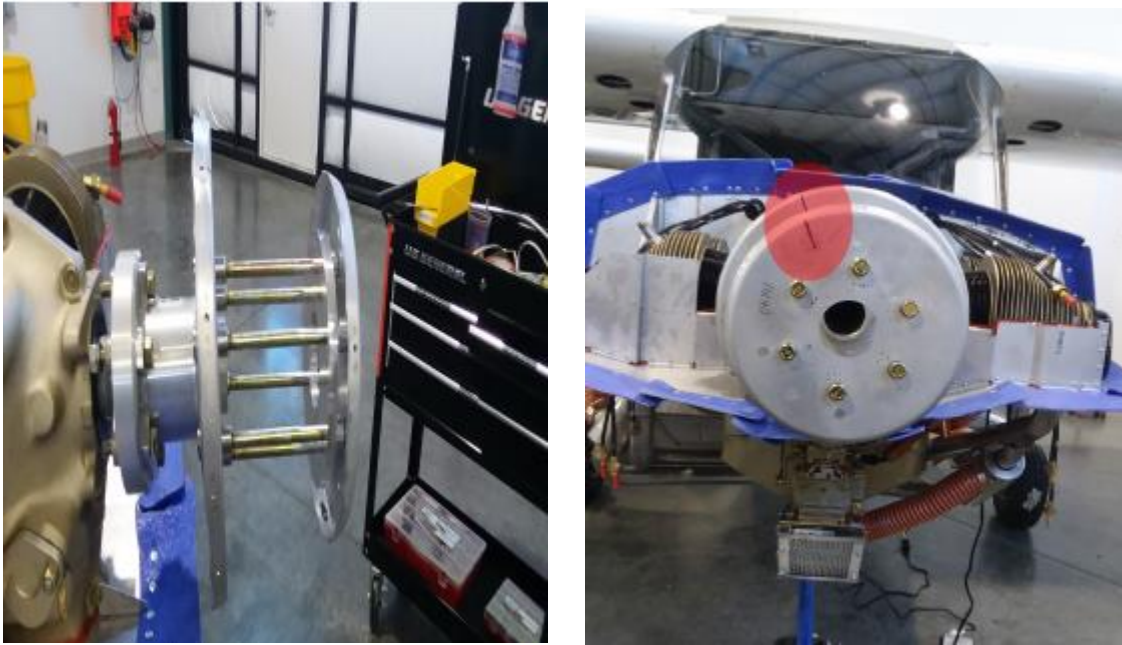
Figure 5.7.16.7 Front spinner bulkhead alignment.
