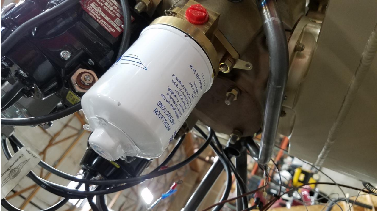
Figure 5.7.10.1 Oil filter secured by safety wire.
